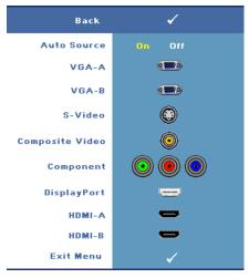
**AUTO SOURCE—**Select On (the default option) to autodetect the available input signals. If you press the Source button when the projector is on, it automatically finds the next available input signal. Select Off to lock the current input signal. If you press the Source button when the Auto Source mode is set to Off, you can manually select the input signal.
